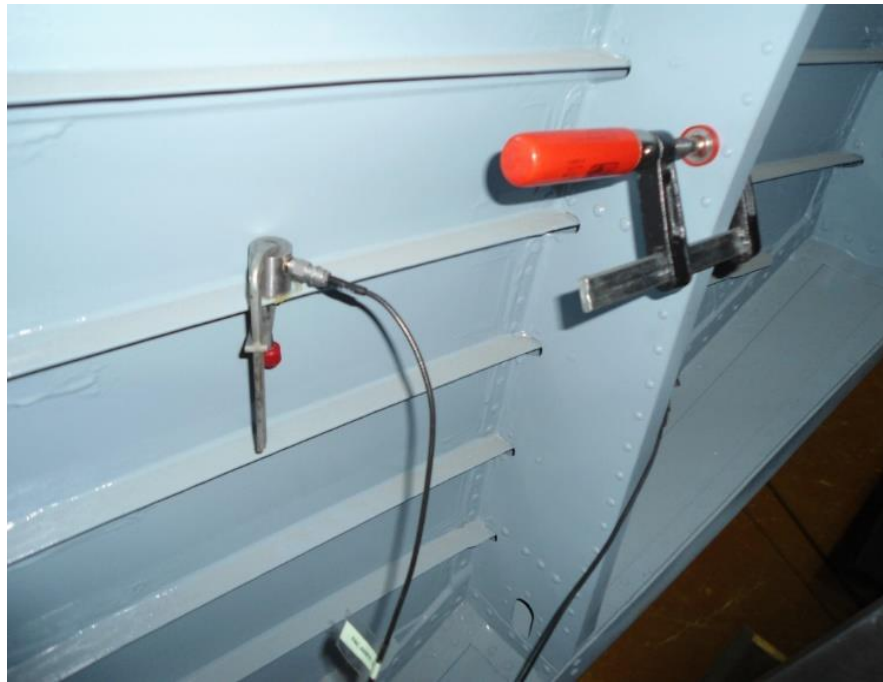
Fig. 1. Location of AE sensors on helicopter fuselage.
