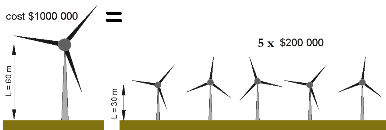
Fig. 1. Comparison of two scale options of wind turbines.
